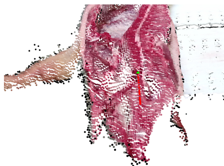
Figure 17. The 5-DoF cutting plane for head cutting illustrated by a green dot and a red normal vector.
