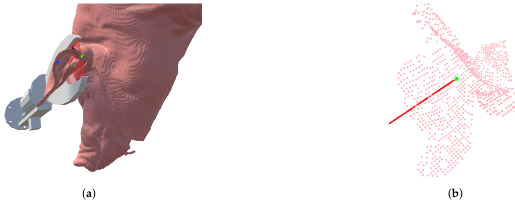
Figure 1. (a) Correct tool pose illustrated using 3D models of the tool and pig. (b) A point cloud of the ear region with our representation of a 5-DoF cutting plane consisting of P_0 (green) and \vec{n}z (red).
