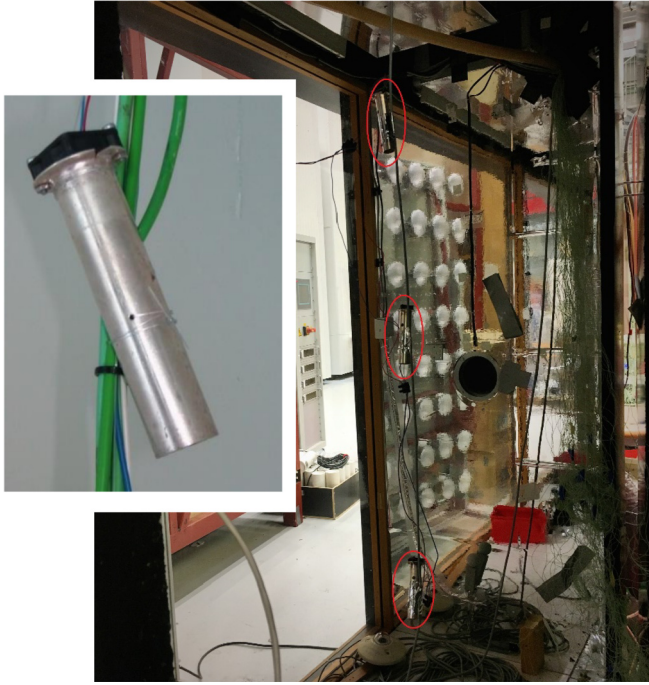
Fig. 6. Measurement of air temperature in the cold box.
