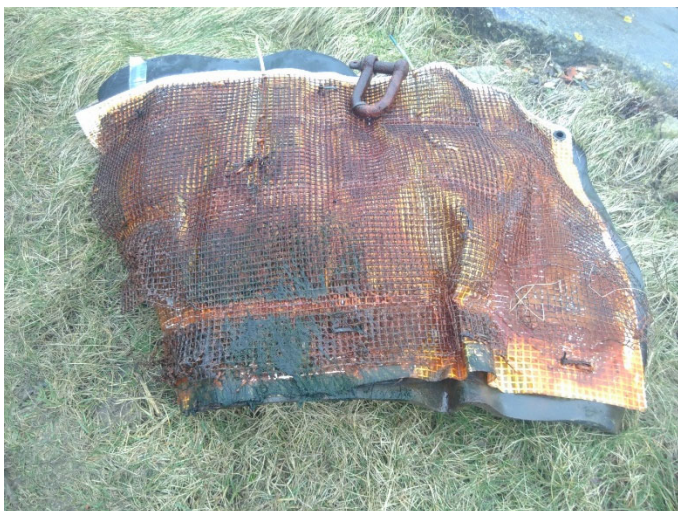
Figure 8. Rusted cathode from Nissum Bredning – after 4 months unprotected at sea.
