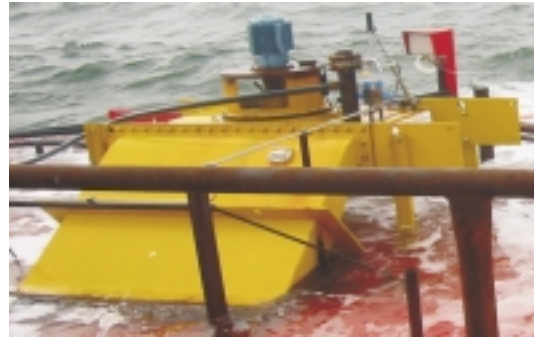
Figure 8: Kaplan turbine with Siphon inlet
