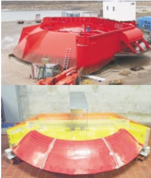
Figure 6: Photo showing the doubly curved ramp.
