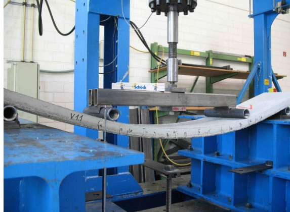
i) Example of FRP reinforcement used in real life concrete structures, ii) Deflected concrete beam with internal GFRP reinforcement.
