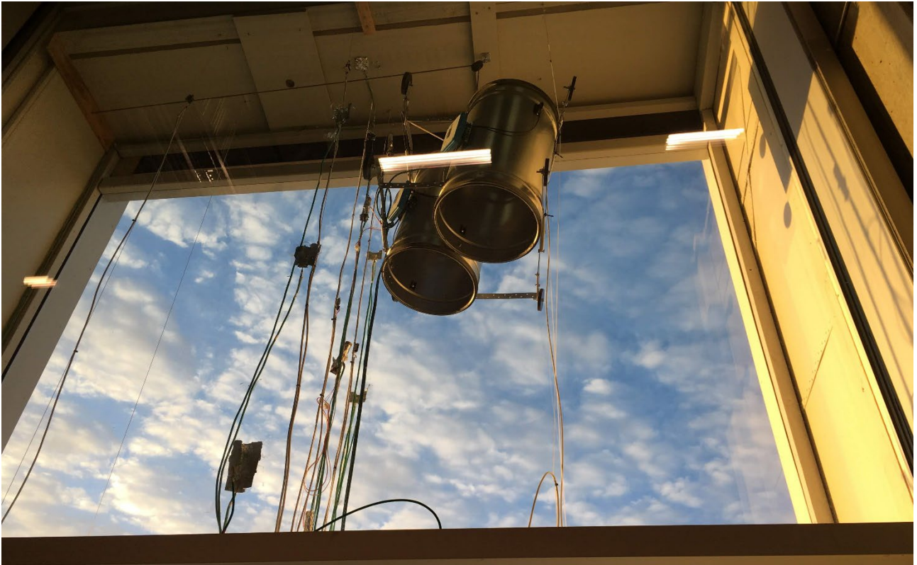
Figure 32: Internal view on the Ultralink air flow sensors (Lindab) in the ventilated cavity of the DSF 23 setup.
