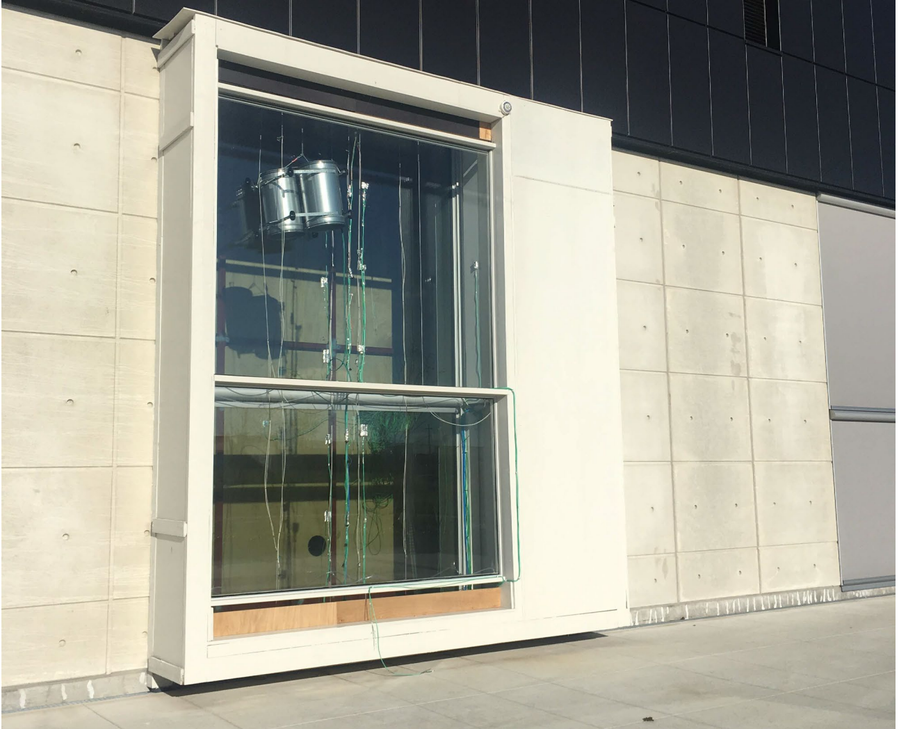
Figure 19: Outside view of the DSF 23 experimental setup.
