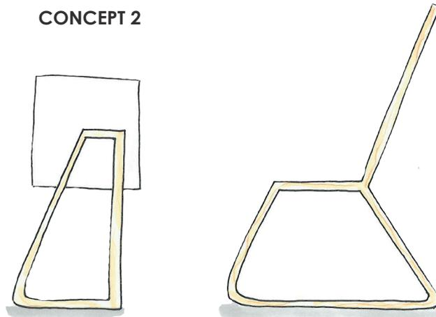
In this concept, the two long sides of the cot are constructed by three parts. The two biggest parts can be tipped over and used as a chair by sliding a flexible bottom plate into the two sides, creating the seat and the back support. Out of the four remaining side parts, two of them can be used as arm support for the chair, and the other two will be used as legs for the bedside crib. The box for the bedside crib is created by the endplates of the cot.
