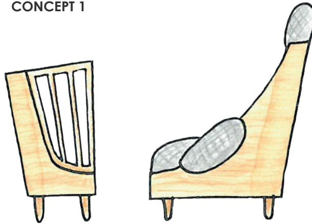
In this shell concept, the cot is split vertically into two pieces. The biggest part is going to be the nursing chair, and the smallest part is the bedside crib. The lats are removed from the chair part, to transform it into a nursing chair. The slope in the top of the cot creates the needed height for the back support, without making it difficult to reach the child in the bed. With the split in the cot, it is possible to extend the bed and turn it into a junior bed.
