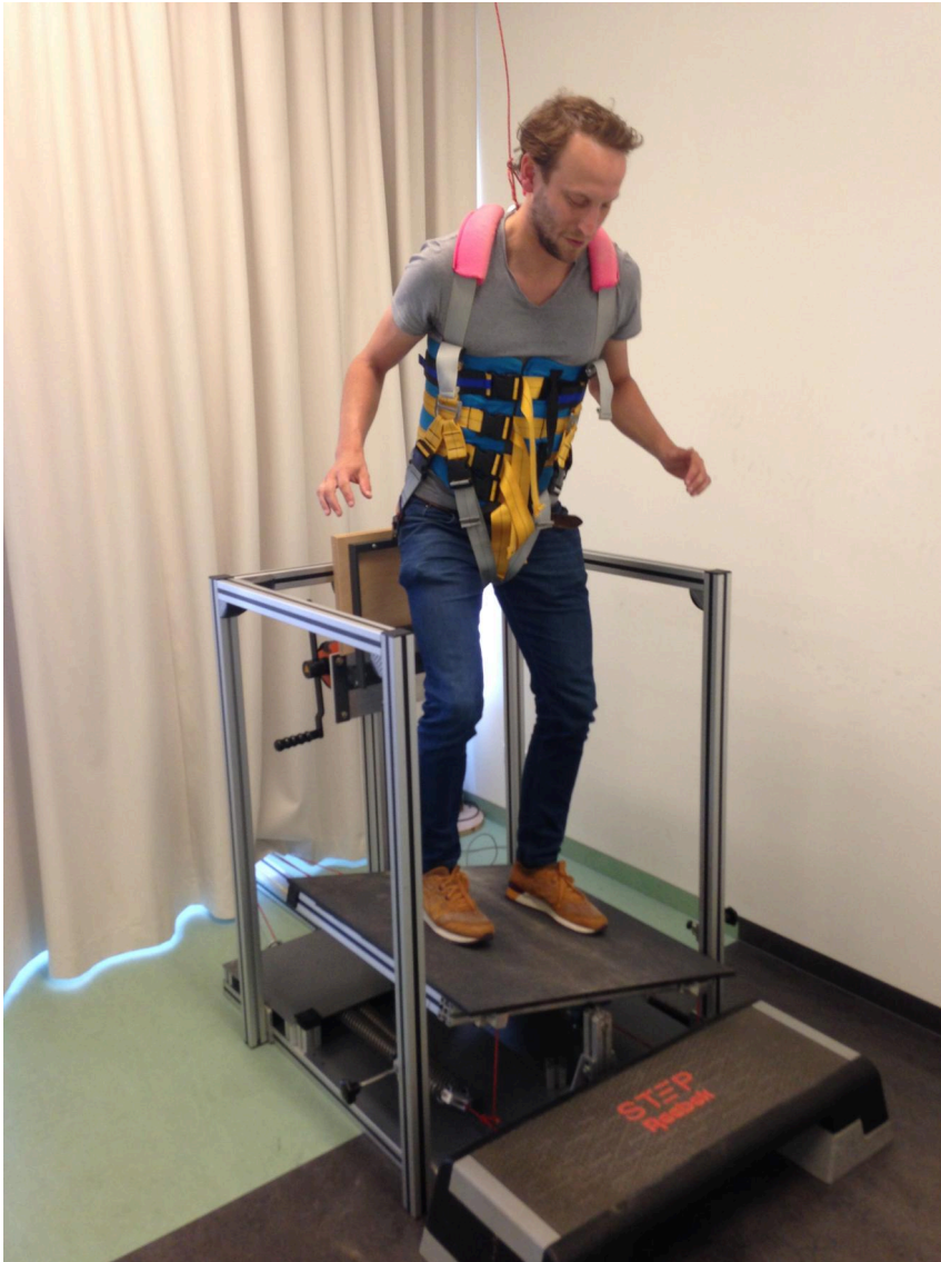
Figure 1. Balance board set-up. Springs were attached to each side of the front of the balance board. Rotational stiffness could be adjusted (0-220 Nm/rad) by using either one or two parallel springs on each side, by altering the springs' moment arm, or by changing the springs themselves (800 N/m vs. 390 N/m). Patients wore a safety harness.
