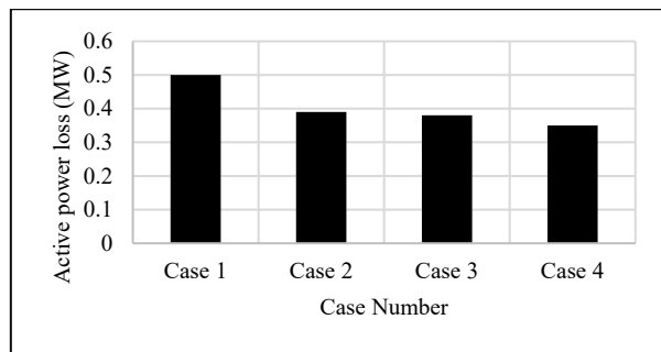
Figure 4-8 Optimized power loss in different cases
