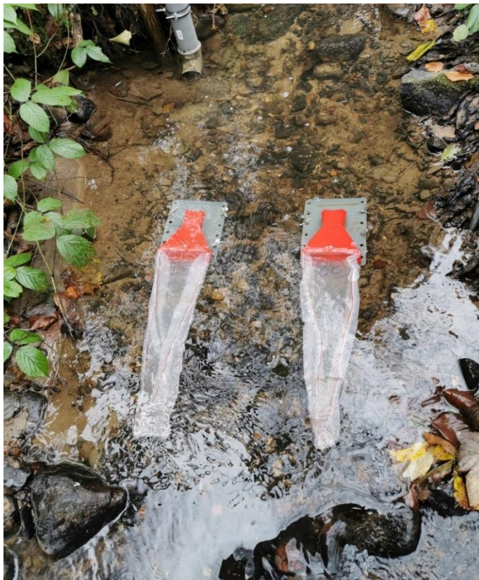
Figure 2.14: Setup of Helley Smith bed sediment samplers in a profile in Polsterbæk.
