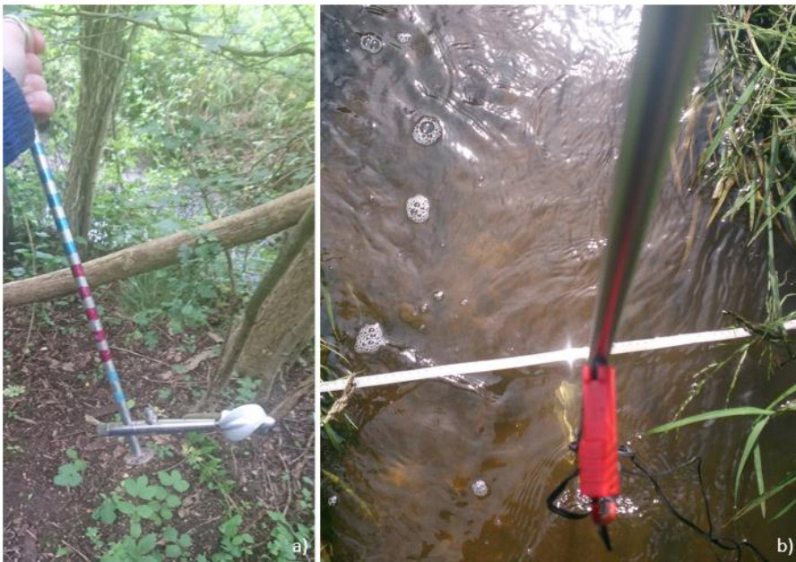
Figure 2.1: OTT C2 flowmeter. a) shows the flow meter with a C6 propeller and b) shows the measurement setup in a stream.
