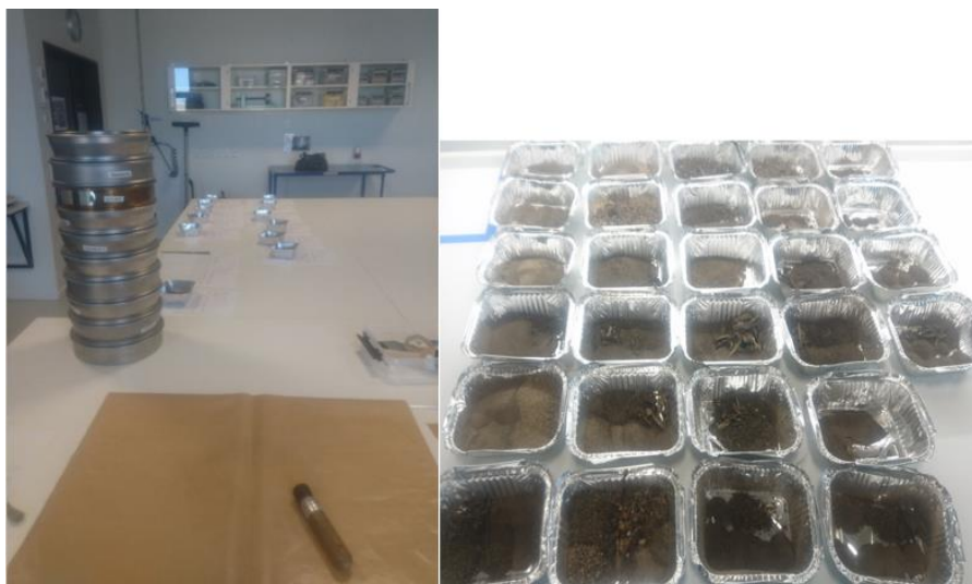
Figure 2.16: a) is the sieving nest used to determine particle size distribution in Paper II , and b) is an example of the sieved samples from the sediment transport experiment.
