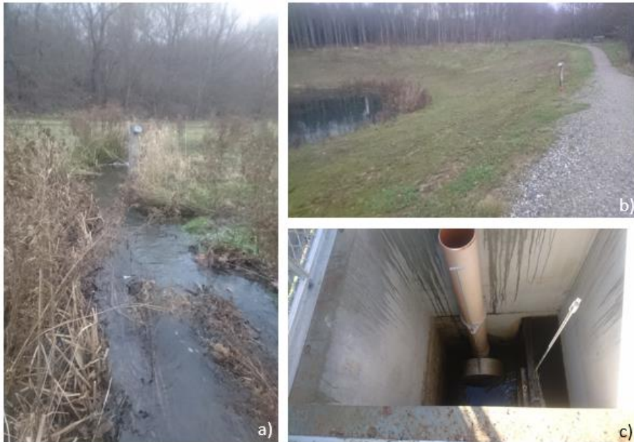
Figure 2.4: Measurement station in Aarhus (Hovedgrøften). a) illustrates the measurement station in the stream Hovedgrøften, and b) illustrates the measurement station in the detention pond which discharges to Hovedgrøften. c) illustrates the water brake in the outlet from the detention pond.
