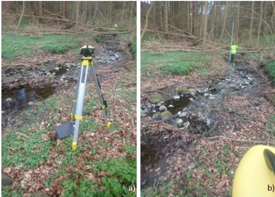
Figure 2.7: Illustration of the equipment for measuring the cross-sections of Polsterbæk. a) shows the electronic levelling device, and b) shows the post used to register the vertical variations in the stream.
