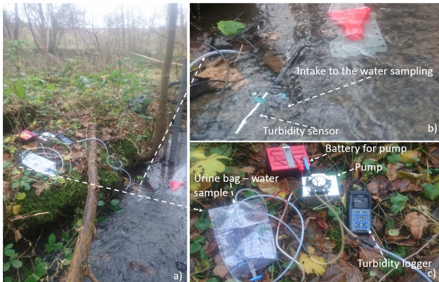
Figure 2.15: Illustration of the experimental setup measuring the suspended sediment transport in Paper II .
