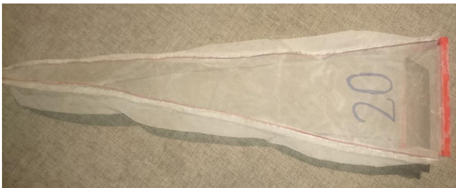
Figure 2.13: One of the sampling bags from the Helley Smith sampler used in the experiments.
