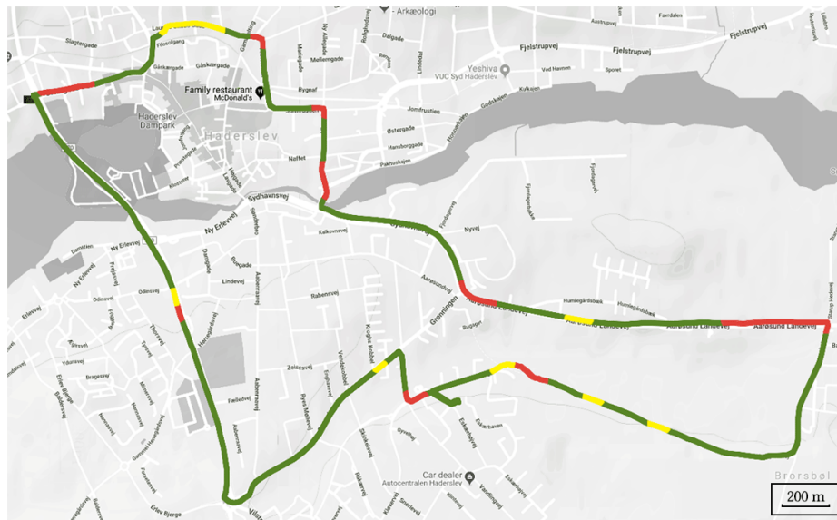
Fig. 2. First route driven by test participant T1, with color coded LowCO 2 (Green), MediumCO 2 (Yellow), and HighCO 2 (Red) peaks.
