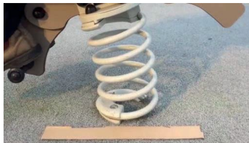
Figure 10: Students measuring the deflection of the spring
