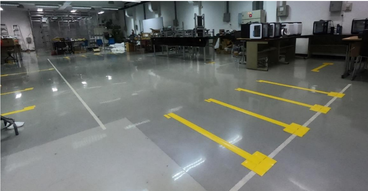
Figure 3: The layout of the Smart Learning Future Factory. The fixed path navigation routes for the AGVs are shown in yellow lines. The open space in the middle allows flexible AGV navigation.
