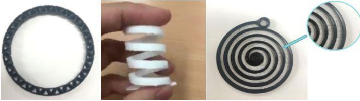
Figure 3. 3D Printed band, compression spring and conical spring
