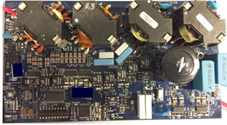
Fig. 6.2: Photo of the PV microinverter product. Source: [J5].
