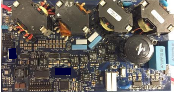
Fig. 2. Photo of the built PV microinverter prototype.
