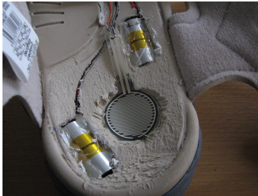
Figure 2: A picture of one pressure sensor and two actuators embedded in the shoes.
