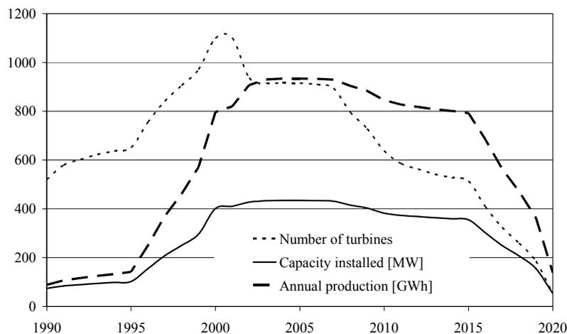
*Figure 1: Projected development of turbine count and capacity in Northern Jutland. If turbines are not replaced after ended technical lifetime of 20 years, there will be a significant decrease in production after 2015.*
