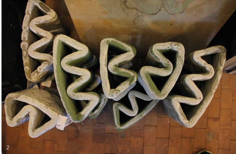
2. Robotically additive-manufactured bricks for the Thermal Tower Project (2018), based on developing thermally-designed concrete composite made through additive manufacturing processes. Photo: MB Jensen (2018).
