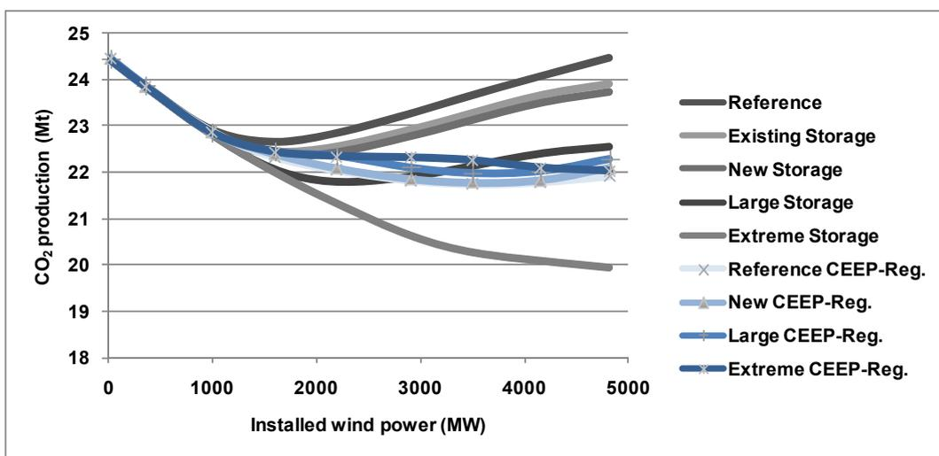
**Figure 2.2.3. CO<sub>2</sub> emissions in the reference energy system with and without PHS and CHP regulation.**
