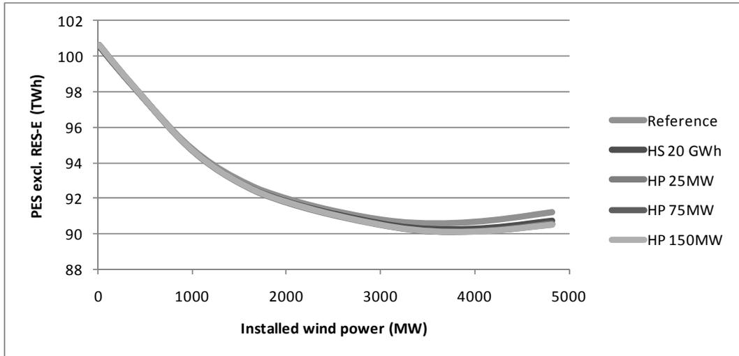
**Figure 2.4.1. Primary energy supply (PES) in a closed energy system analysis of the reference energy system with and without heat storages, heat pumps and CHP regulation.**
