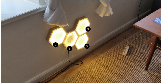
Figure 1: The Lumen physical ambient light displayed in a participating household. 1) The centre hexagon cover lights up to display that the current electricity is considered sustainable. 2) This cover illustrates that the current household is using electricity. 3) These two covers show, which other households in the community are using electricity sustainably.
