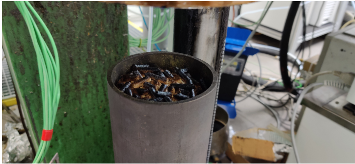
Fig. 4.7: The bed surface after two hours pyrolysis with \text{N}_2 at PF 30 \text{ l min}^{-1}
