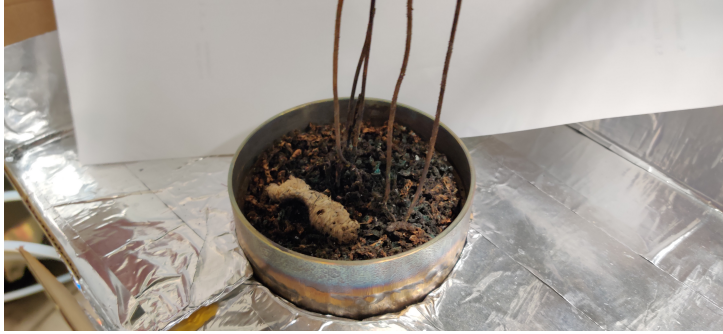
Fig. 4.6: Ashes after combustion under PF 30 \text{ l min}^{-1}
