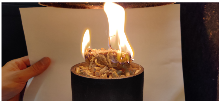
Fig. 4.5: Ignition packed bed with an ignitor
