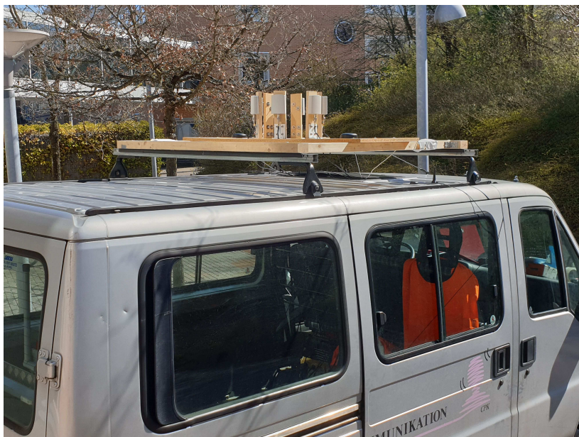
Fig. F.2: A measurement vehicle with the antenna structure on the roof
