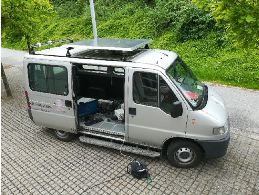
Fig. D.2: A van with measurement equipment (inside) and antenna array mounted on a ground plane (roof)
