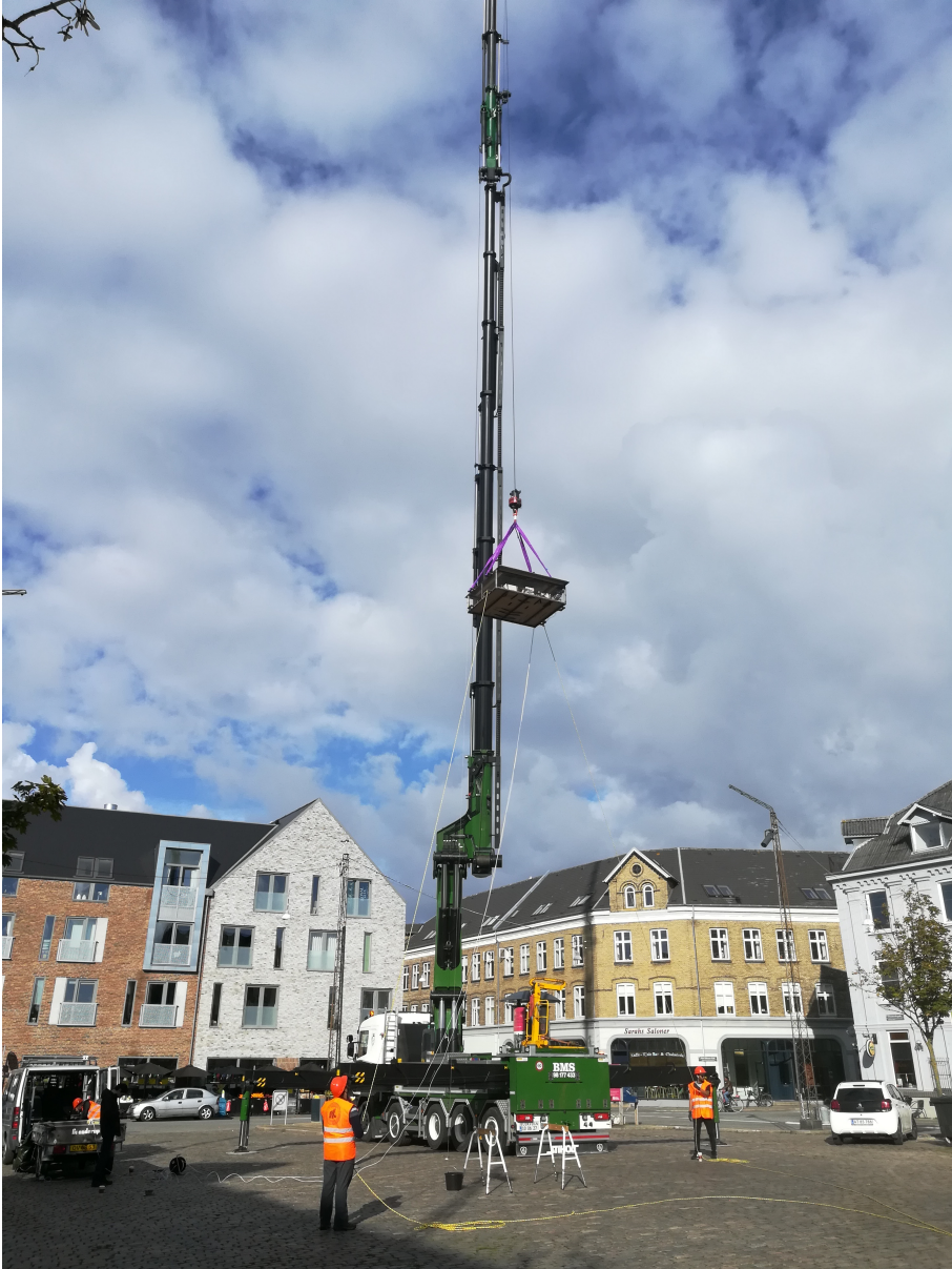
Fig. A.14: Designed testbed lifted in the air during measurement campaign focusing on a UAV A2G channel characterization
