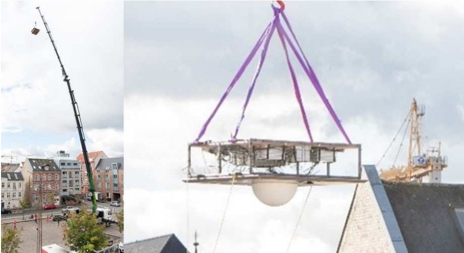
Fig. B.2: Assembled setup lifted to 40 meters high by a crane (left) and zoomed (right)
