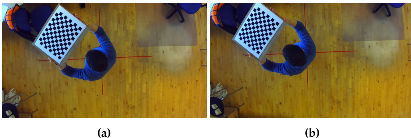
Fig. 1.1: Examples of (a) left and (b) right image from the ZED camera used for calibration.
