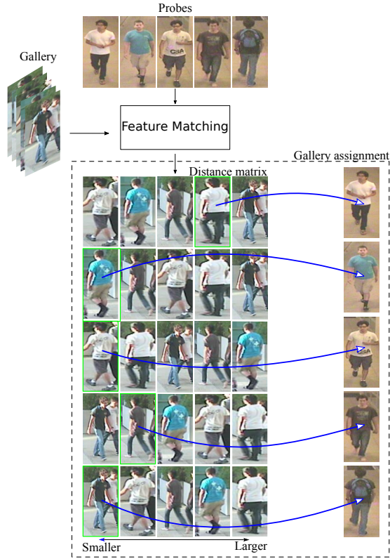
Fig. F.2: Overview of the assignment procedure. We match each probe against all gallery features to produce initial lists based on likelihood, which is defined by distances. Images further to the left have smaller distances to the probes and vice versa, while green boxes indicate true matches. Afterwards, the Hungarian algorithm [7] is applied to assign each gallery to only one of the probes by minimizing the total distance.
