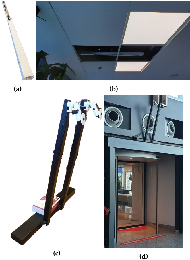
Fig. 3.1: (a) The camera mount used at the entrance and (b) the corresponding placement in the ceiling along with the two extra LED light sources. (c) The camera mount used at the exit and (d) the placement of the mount above the exit.
