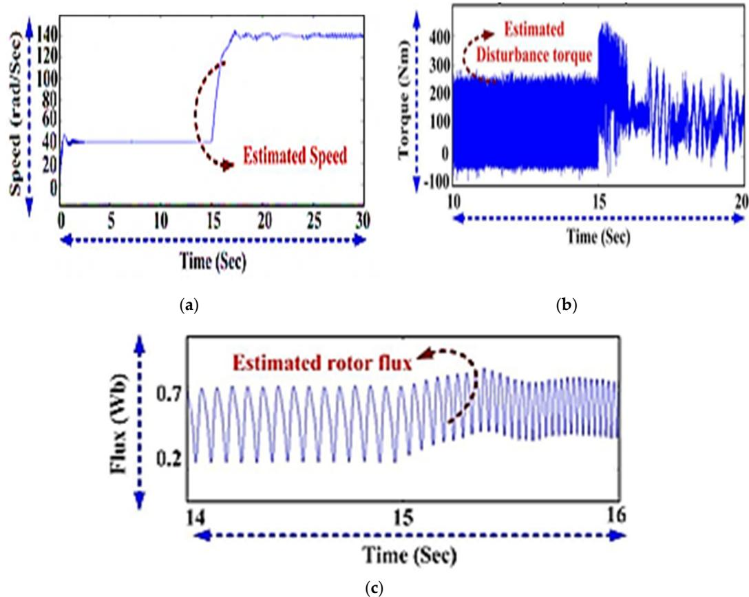
**Figure 9.** SMLO1: (a) estimated speed; (b) estimated torque and (c) estimated rotor flux.
