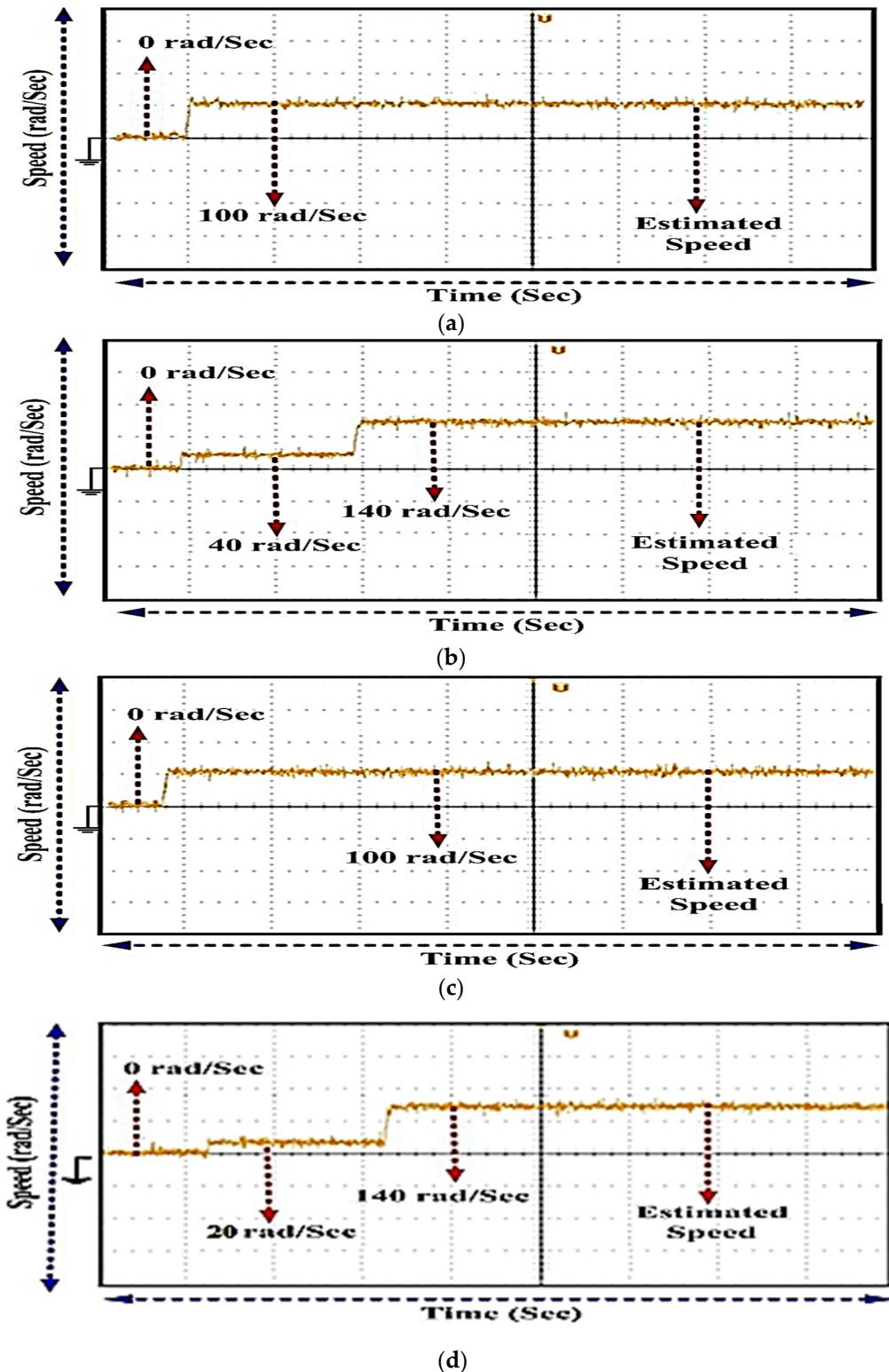
**Figure 16.** Estimated speed: (a) for a constant speed reference of 100 rad/s for SMLO1, (b) for a step speed reference of 40–140 rad/s for SMLO1, (c) for a constant speed reference of 100 rad/s for SMLO2 and (d) for a step speed reference of 20–140 rad/s for SMLO2.
