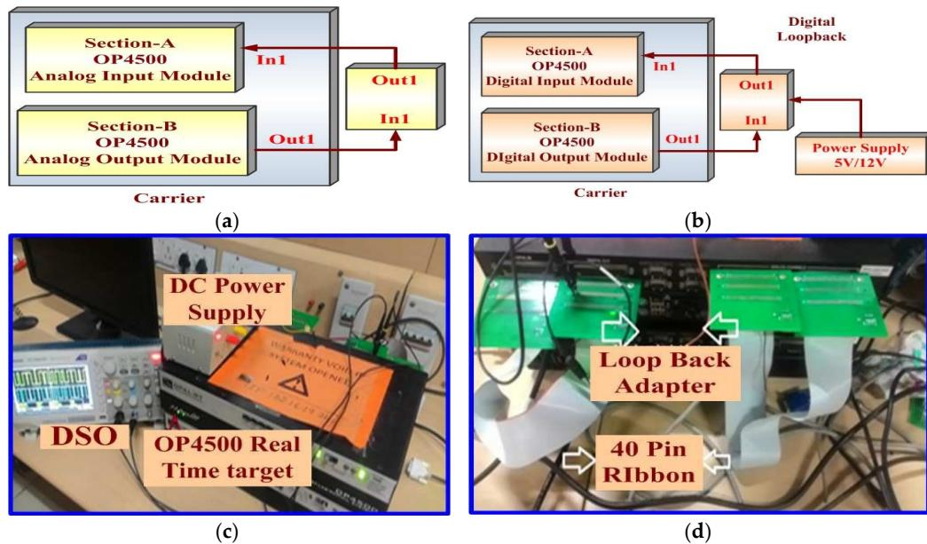
**Figure 3.** Representation of real-time PIL test bench using OP4500: (a) analog loopback; (b) digital loopback; (c) OP4500 target and power supply for digital loopback and (d) rear view of OP4500 with analog and digital loopback.
