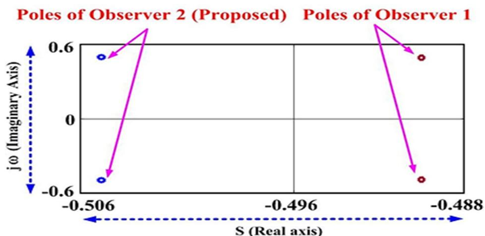
**Figure 17.** Pole placement of SMLO1 and SMLO2.
