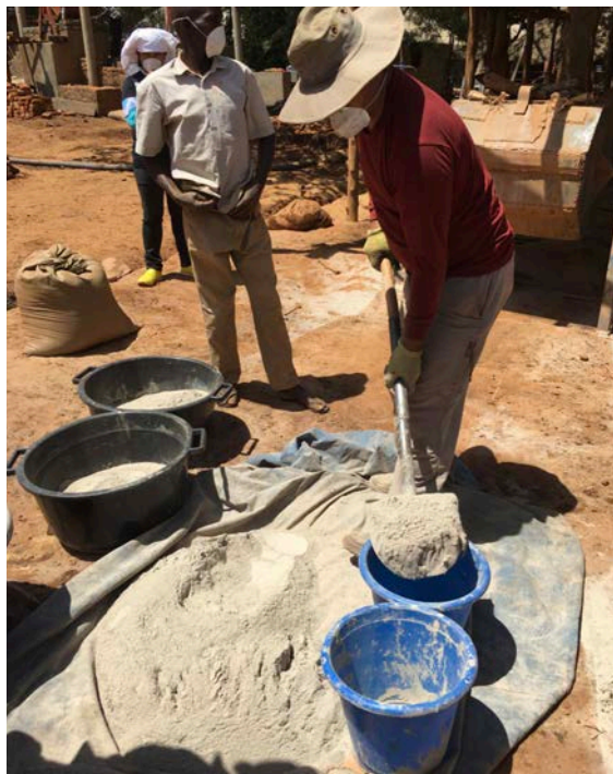
Figure 5 — The dry milled ore is divided spade by spade into two lots. Published with permission.
