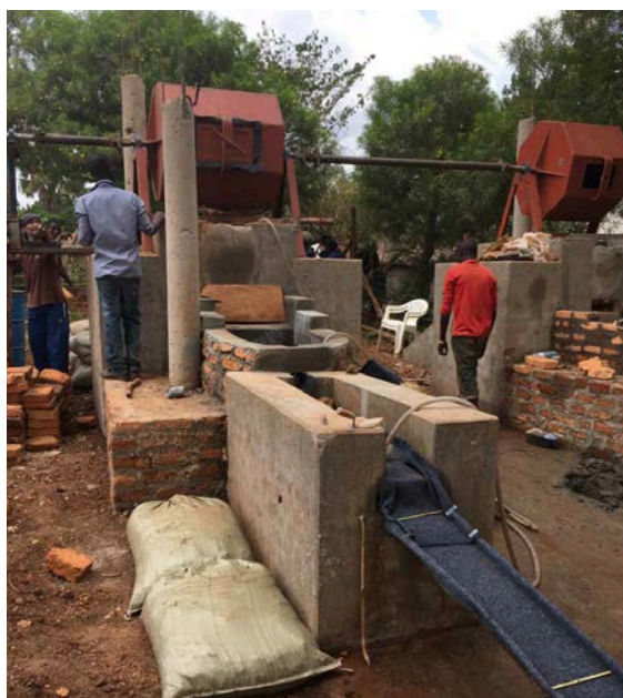
Figure 3 — Processing station built as part of the project to process gold with direct smelting. Two interconnected ball mills followed by two successive sluice boxes and a launder. Published with permission.
