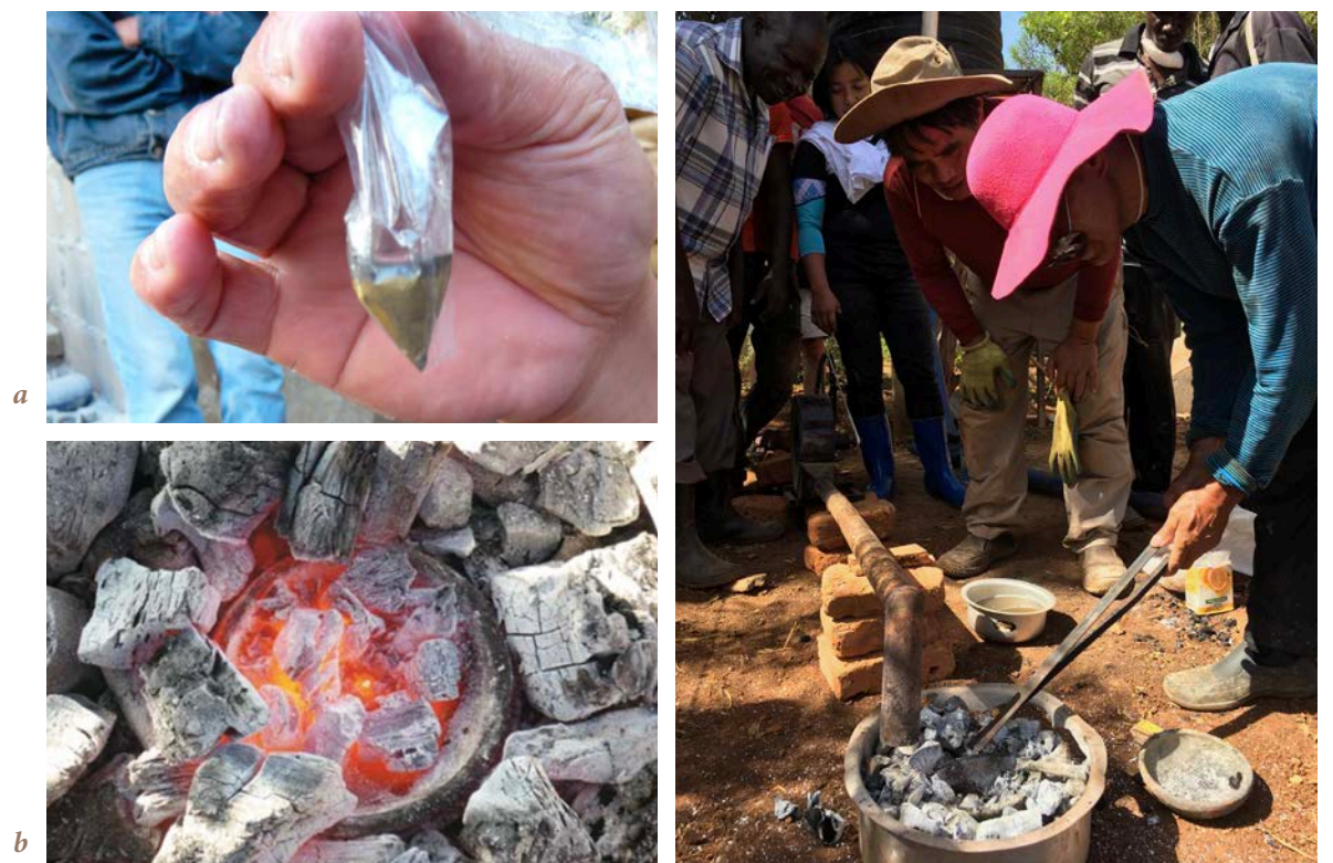
Figure 4 — a) Plastic bag with gold concentrate, borax and a few drops of water. b) Clay ball with molten gold in the center. c) Smelting of the gold concentrate. Published with permission.
