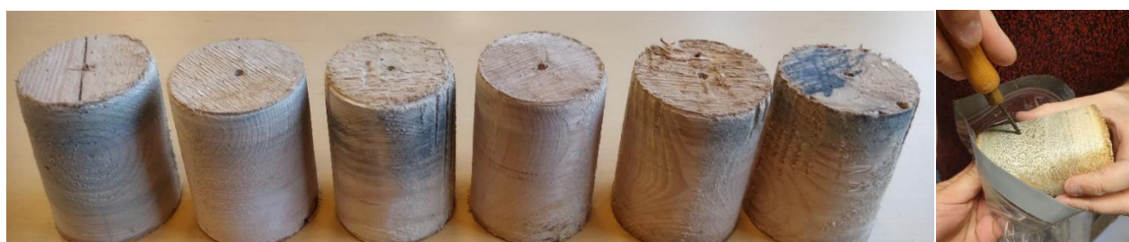
Fig. 8. Left: The 6 specimens drilled out from the supportive wall plates from the 6 wall configurations; left to right: X1, X2, X8, G1, G4, G5. Right: awl test of a specimen.
