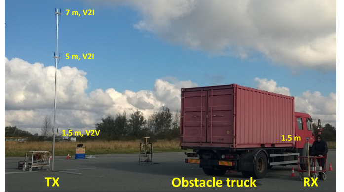
Fig. 1. Measurement scenario and setup with stationary TXs deployed at 1.5 m (V2V configuration), 5 and 7 m (V2I configuration), large vehicle obstacle (truck), and moving RX at 1.5 m.
