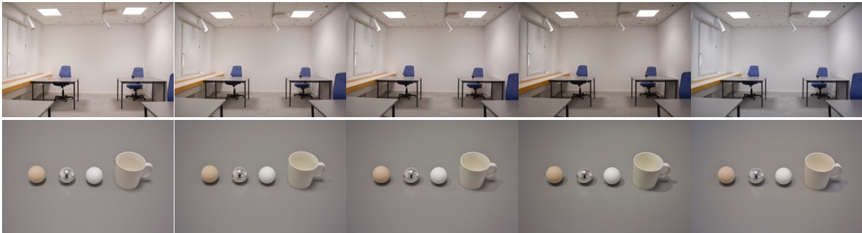
Ill. 1. Ex1 lighting scenarios from left: 1.1, 1.2, 1.3, 1.4 and 1.5, illustrating the light distribution and perceived CCTs of the space and of objects on a work desk.
