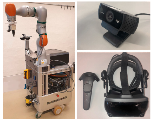
Fig. 3. Hardware components of the system: Mobile manipulator platform (left), one instance of the Logitech C922 webcam (top-right), Valve Index VR headset and the HTC VIVE VR controller (bottom-right).
