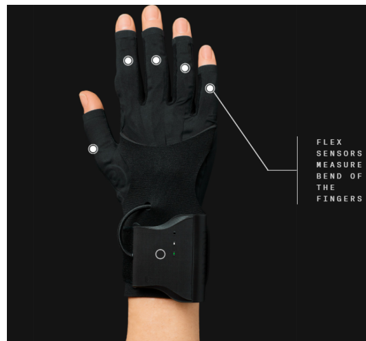
Figure 1.1: A MI.MU glove, taken from [17].
