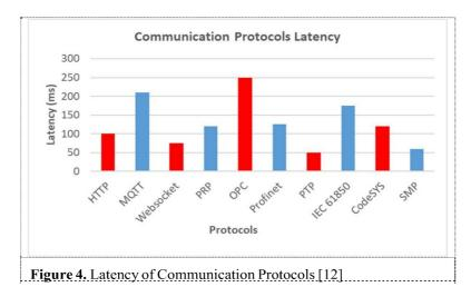
The reason for the lower latency in the SMP when compared to WebSocket and OPC, is due to the lack of acknowledgement and checksum fields in the SMP protocol. Since the OPC has redundant acknowledgment fields and waits for returns on the original message, scaling networks with use of OPC
