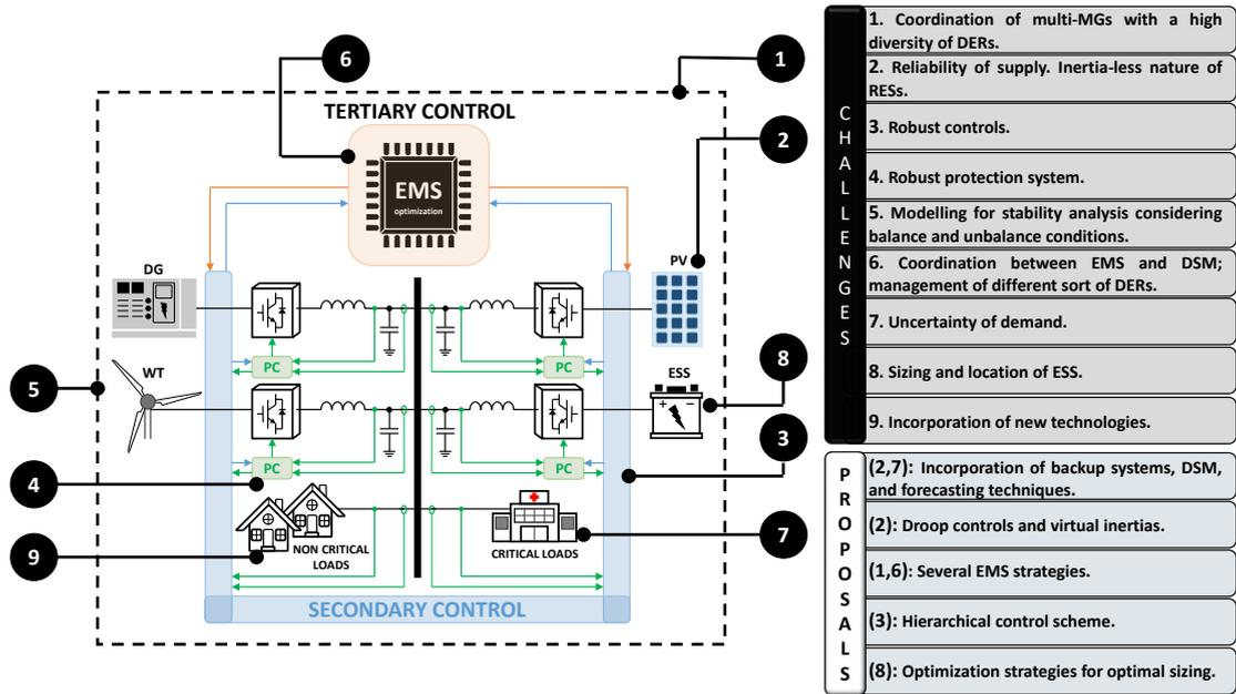
**Fig. 1:** A generic IMG with some current challenges and solutions proposed in the literature. Green lines: primary control communication. Blue lines: secondary control communication. Orange lines: tertiary control communication.
