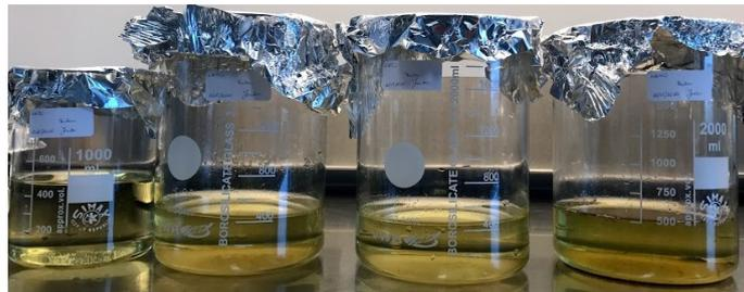
(b) Outlet water samples and blank sample - After Fenton oxidation
