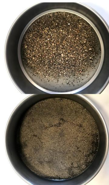
(b) The larger and the smaller than 1 mm sample fractions (LS4T)
