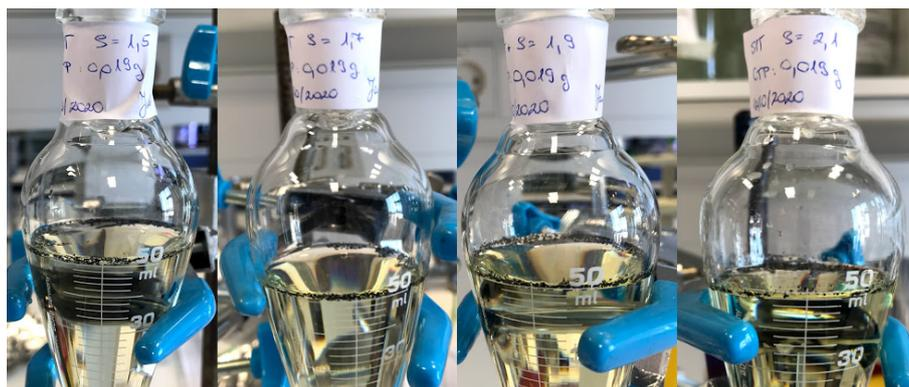
Figure 3.7: Car tire density experiment. The density values from left to right:  $1.5 \text{ g} \cdot \text{m}^{-3}$ ,  $1.7 \text{ g} \cdot \text{m}^{-3}$ ,  $1.9 \text{ g} \cdot \text{m}^{-3}$ ,  $2.1 \text{ g} \cdot \text{m}^{-3}$
