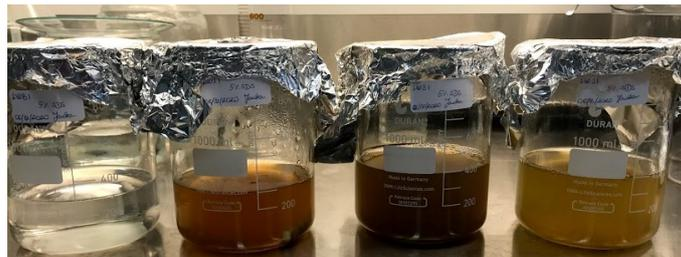
(a) Inlet water samples and blank sample - After SDS treatment
