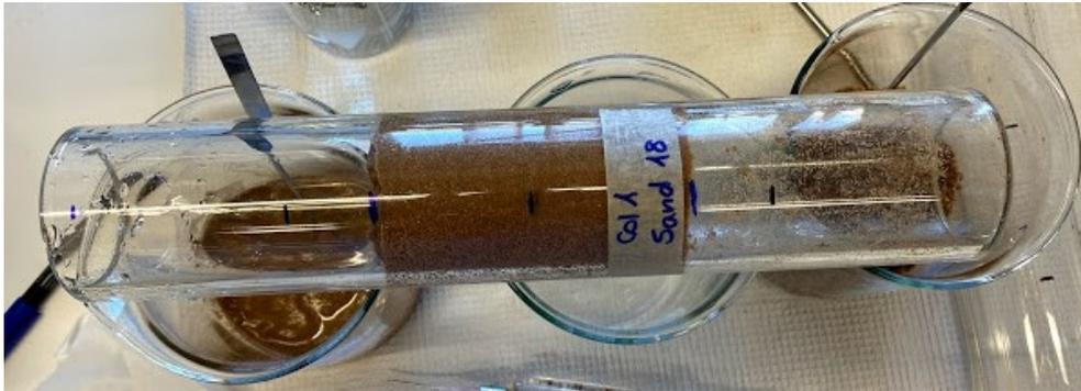
Figure 6.3: Divide the amount of soil in the column into three parts
