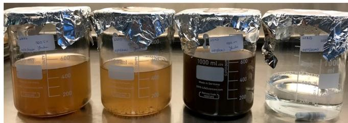
(b) Outlet water samples and blank sample - After SDS treatment
