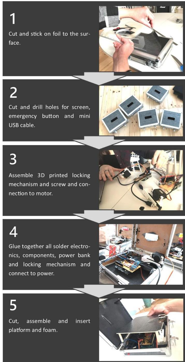
Figure 4.6. Assemble Process.
