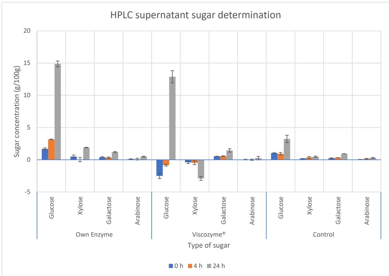
Figure 23: HPLC result of the sugar concentration in the supernatant after the second filtration.
