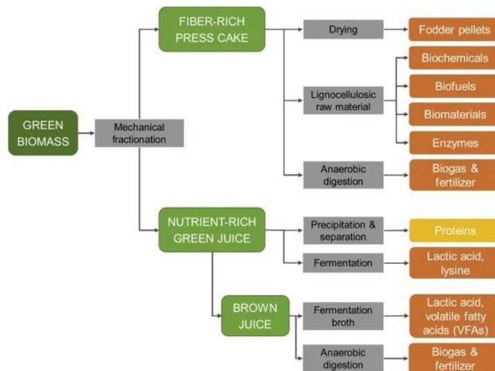
Figure 2: Schematic diagram for potential uses for the three fractions: green juice, brown juice, and press cake (Santamaría-Fernández et al., 2020).
