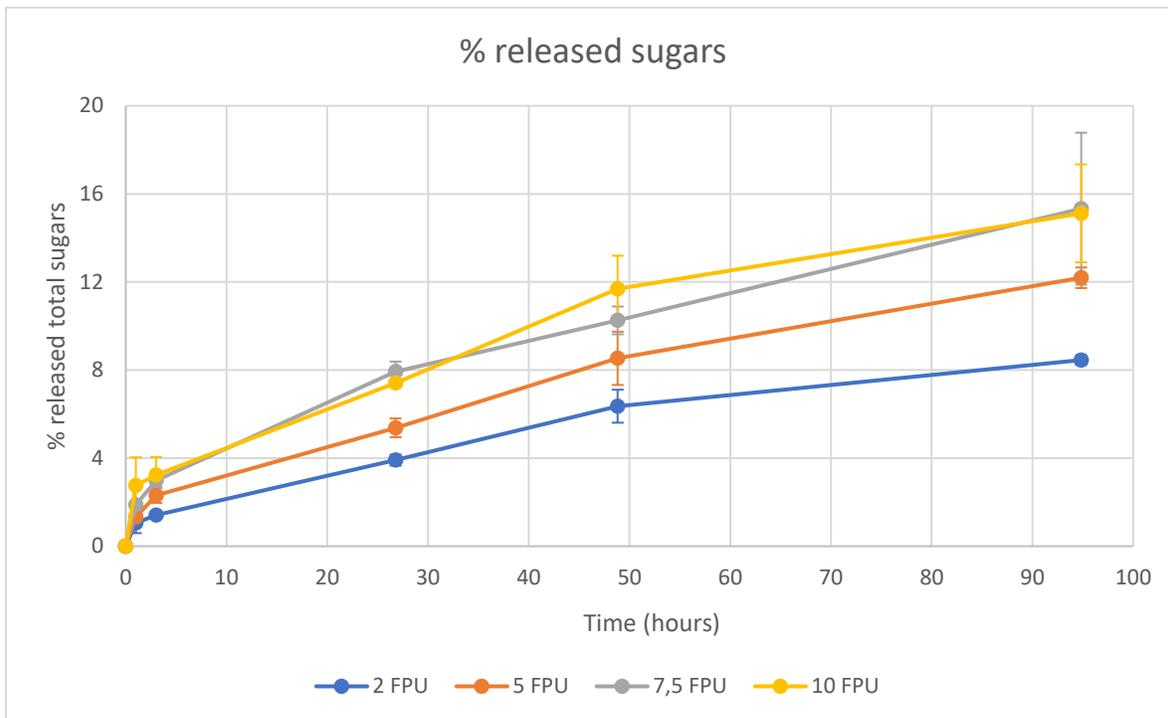
Figure 18: Optimization of the enzymatic hydrolysis in the experiment "time/units". Blue represents 2 FPU/g-DM substrate, Orange represents 5 FPU/g-DM substrate, Gray represents 7.5 FPU/g-DM substrate, Yellow represents 10 FPU/g-DM substrate.
