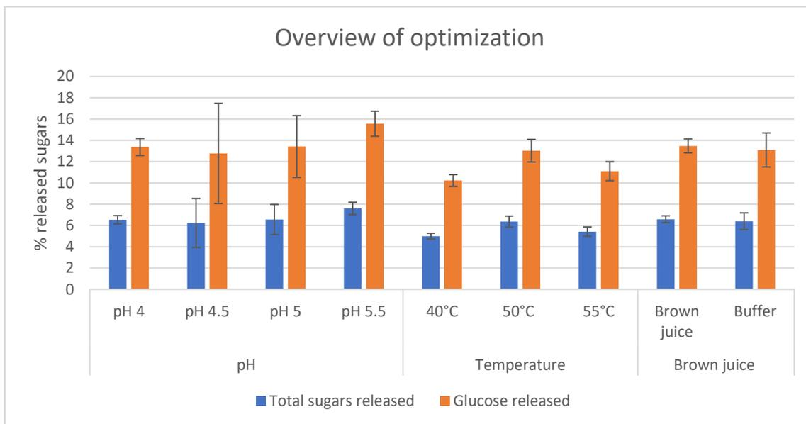
Figure 19: Optimization of the enzymatic hydrolysis in the experiments “pH”, “temperature”, and “brown juice”. Blue blocks represent the % of released sugars if both cellulose and hemicellulose is degraded. Orange blocks represent the % of released sugars if only cellulose are degraded.
