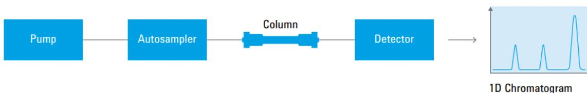
Figure 6: Simple box diagram of a HPLC procedure (Agilent Technologies 2016).
