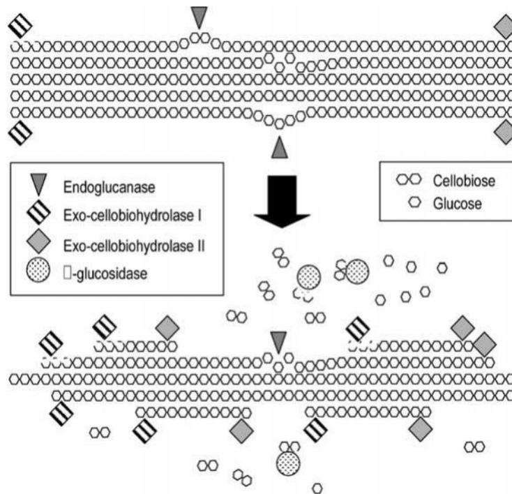
Figure 3: Hydrolysis of cellulose using the different cellulases (Malherbe and Cloete, 2002).
