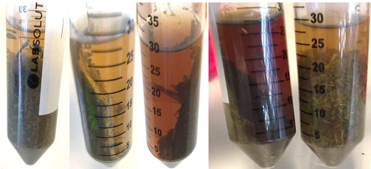
Figure 11: Content of flasks after centrifugation. From the left: after 0 days of incubation, after 5 days of incubation, after 9 days of incubation, after 14 days of incubation, where the tube to the right is the control.
