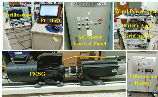
Figure 15. Configuration of the experimental DCMG system.
