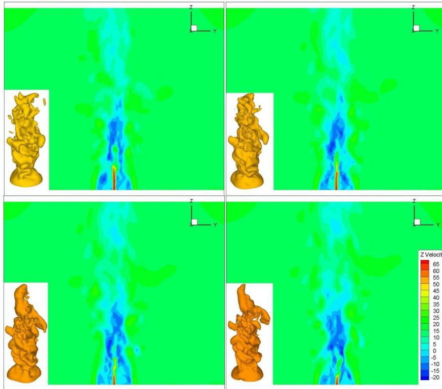
Figure 7: Isosurface of pressure and contour of axial velocity from  $t=0.171s$  to  $t=0.178s$
