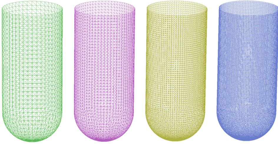
FIGURE 3 Four different mesh resolutions of floating body used for non-linear WEC-Sim simulation (left to right: coarse to extra fine)
