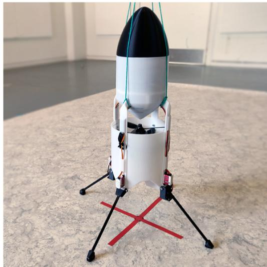
**Figure 7.4:** 4-DOF setup ( $x$  and  $y$  restricted) used to evaluate the control of altitude.
