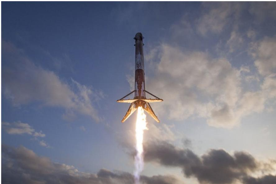
**Figure 1.1:** Reentry of the Falcon 9 rocket, performing a controlled vertical landing [3]
