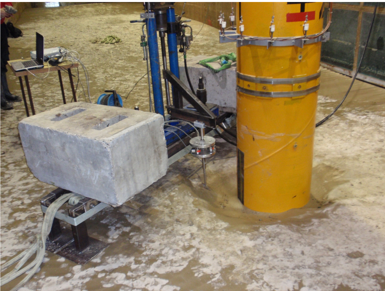
Figure 4: Taking cone penetration tests of the soil after the generation of waves and drainage of water. The size of the scour hole after the waves can also be observed.
