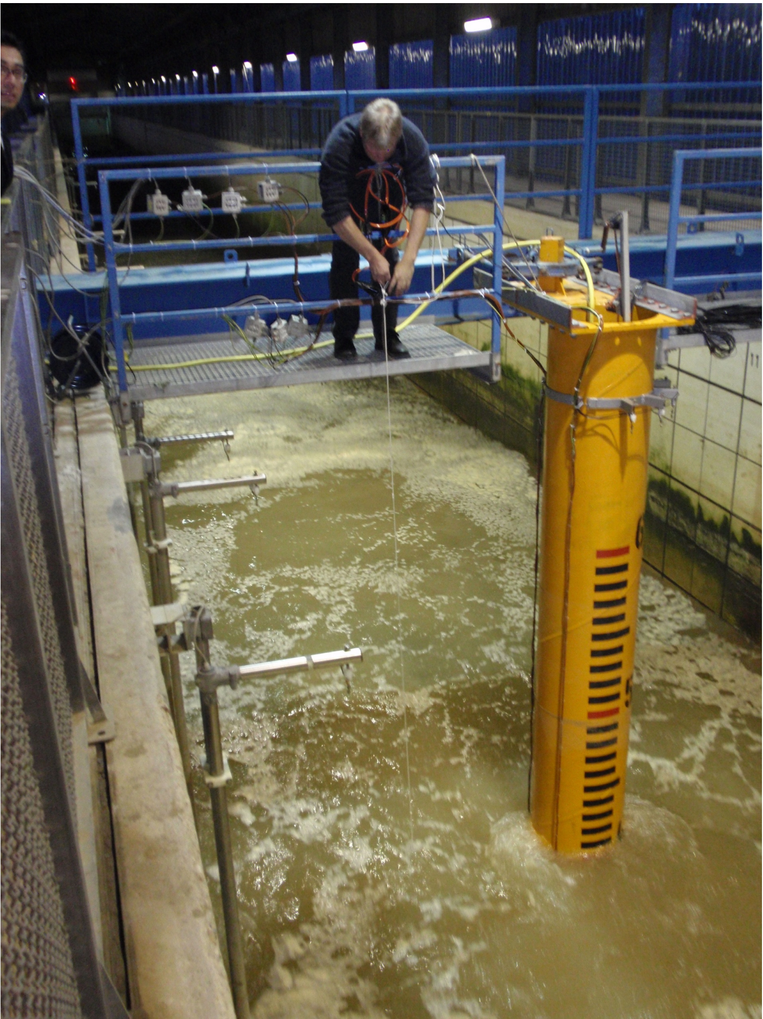
Figure 5: Running of waves and continuous measurement of scour depth.
