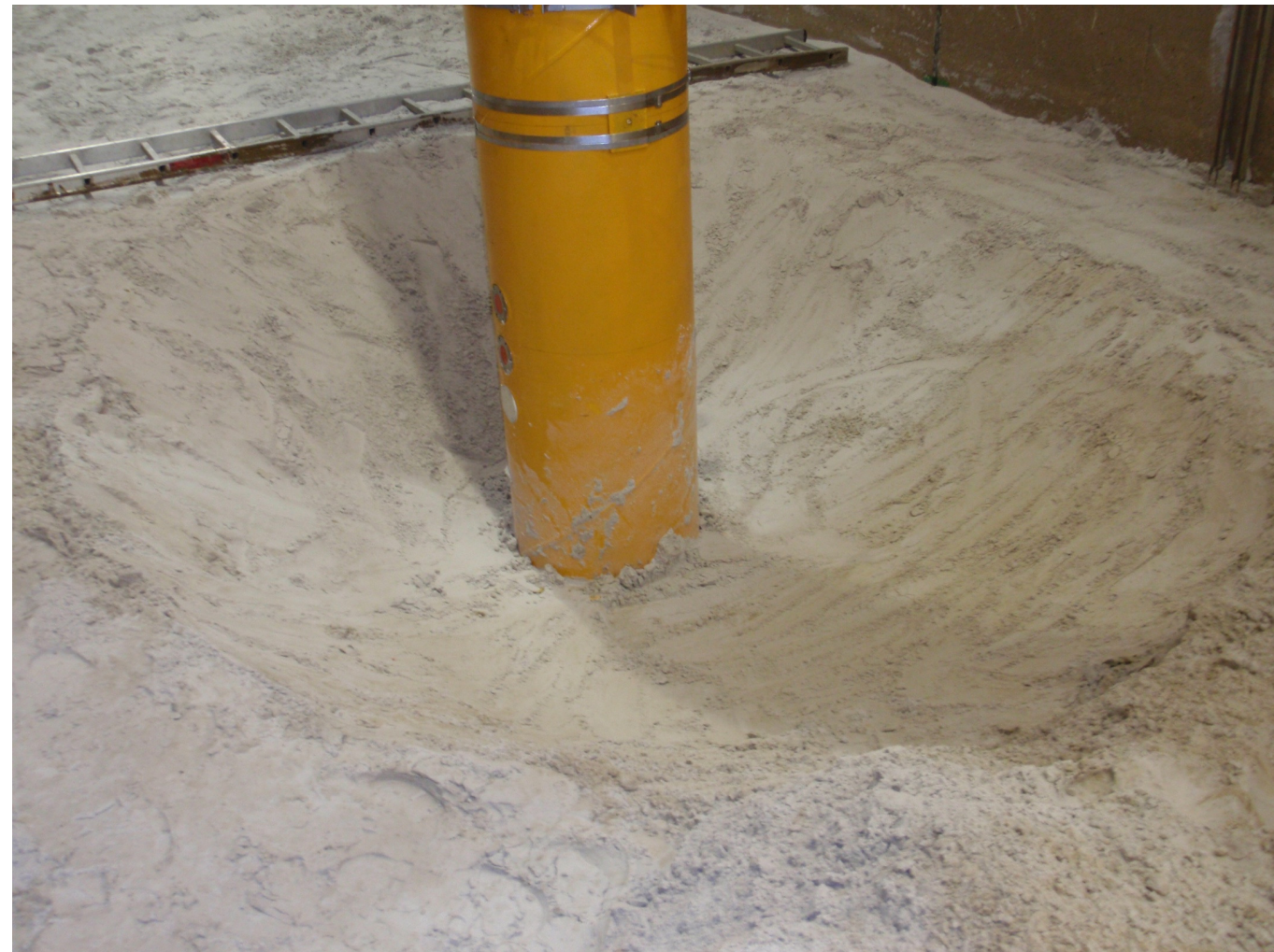
Figure 2: Manually prepared scour hole.
