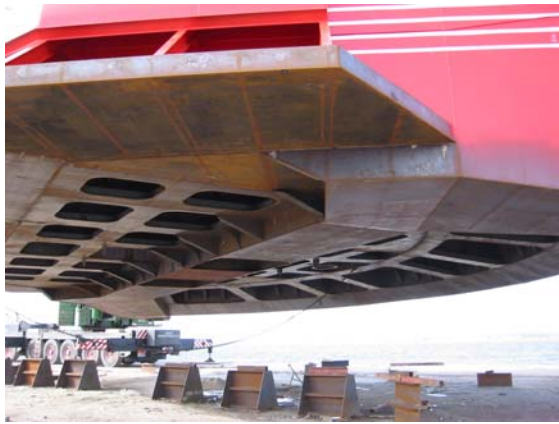
Figure 7: The open air chambers can not be modelled in small scale testing.
