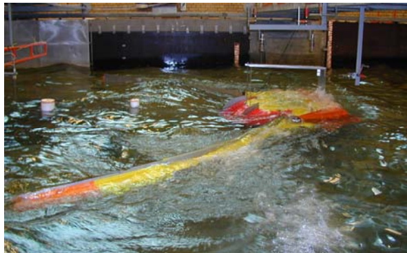
Figure 8: In high sea states the Wave Dragon just allows the waves to spill over.
