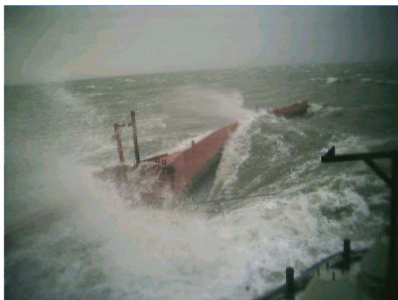
Figure 9: Over spill at the prototype during a storm with wind speed of 25 m/sec.
