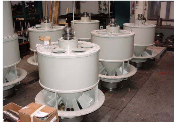
Figure 12: The six axial propeller turbines being assembled at Kössler GmbH
