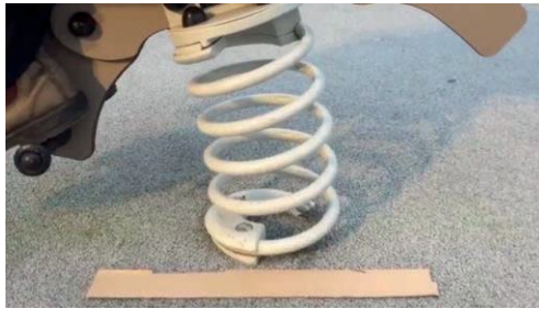
Figure 10: Students measuring the deflection of the spring
