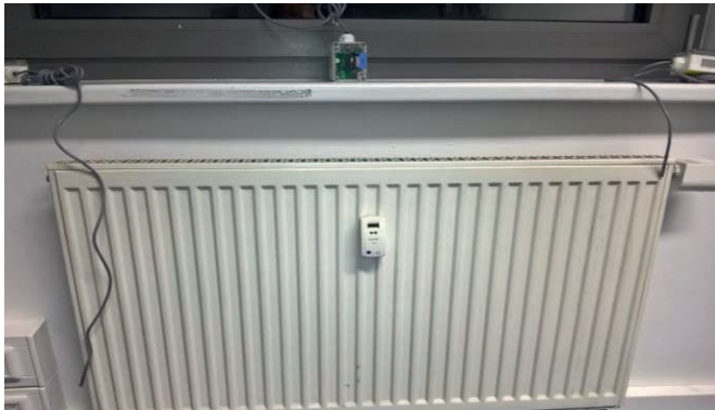
Figure 4: Measurement points at radiators
