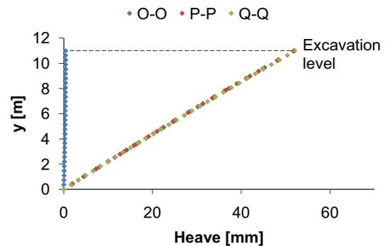
**Figure 16:** Vertical displacements through the cross-sections O-O through Q-Q.  $y = 0$  m is the lower horizontal boundary of the model and  $y = 11$  m is the level of the pile head, i.e. the excavation level.
