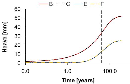
**Figure 27:** Heave at the points B, D, E and F as a function of time. The dashed line indicates 40 years, i.e. the time at which the heave in the pile starts to decrease.
