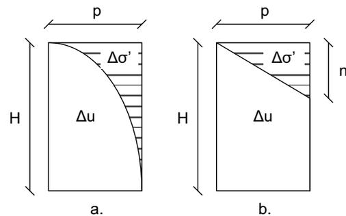
**Figure 4:** Stress variation for consolidation with one-sided drainage where  $H$  is the height of the layer,  $p$  the unloading pressure,  $\Delta u$  the excess pore pressure and  $\Delta\sigma'$  the effective stress variation. a. One-sided drainage by Terzaghi's theory of consolidation. b. Linear approximation where  $n$  is the height of the swelling zone.
