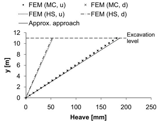
**Figure 12:** Heave calculated by PLAXIS (*FEM*) and the approximative approach of Eq. 7 through the axis of symmetry.  $y = 0$  is the lower horizontal boundary of the model.  $u$  is for undrained and  $d$  for drained strength parameters.
