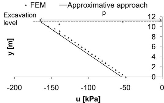
**Figure 11:** Pore pressures calculated by PLAXIS and the approximative approach of  $\gamma_w$ ,  $\Delta u$  and the depth through the axis of symmetry.  $y = 0$  is the lower horizontal boundary of the model.  $p = \gamma_{unsat} \cdot 10 \text{ m}$  is the unloading pressure.
