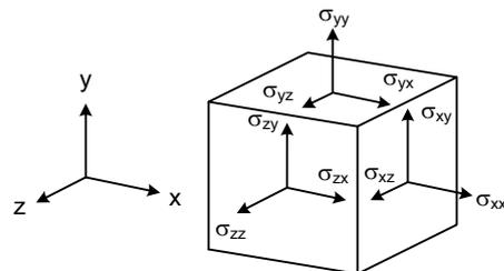
**Figure 2:** Coordinate system and sign convention of stresses.
