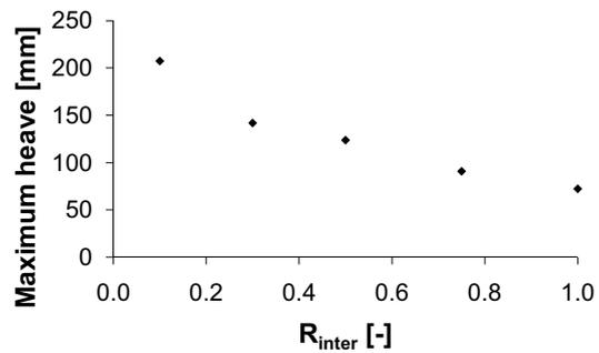
**Figure 7:** Maximum heave of the excavation level as a function of the strength reduction factor  $R_{inter}$ .
