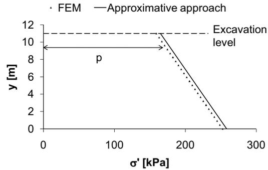
**Figure 10:** Effective stresses calculated by PLAXIS and the approximative approach of  $\gamma'$  and the depth through the axis of symmetry.  $y = 0$  is the lower horizontal boundary of the model.  $p = \gamma_{unsat} \cdot 10 \text{ m}$  is the unloading pressure.
