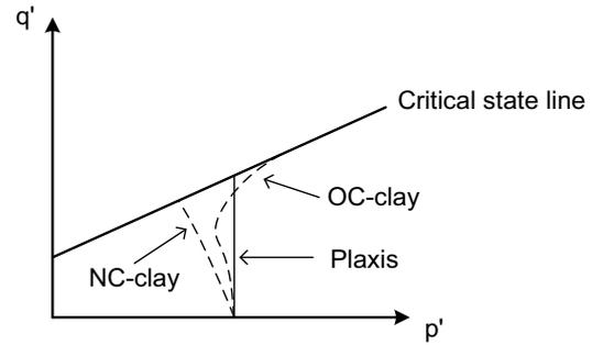
**Figure 8:** Effective stress paths for normally consolidated clay (NC-clay), overconsolidated clay (OC-clay) and for an undrained Mohr-Coulomb material with drained strength parameters defined in PLAXIS (Plaxis).
