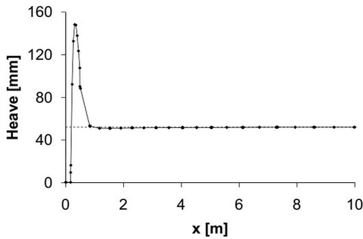
**Figure 17:** Heave through the cross-section Q-Q, i.e. at the excavation level.  $x = 0 \text{ m}$  is the axis of symmetry and  $x = 10 \text{ m}$  is the right vertical boundary of the model. The dashed line indicates the heave of the excavation level at the right vertical boundary.
