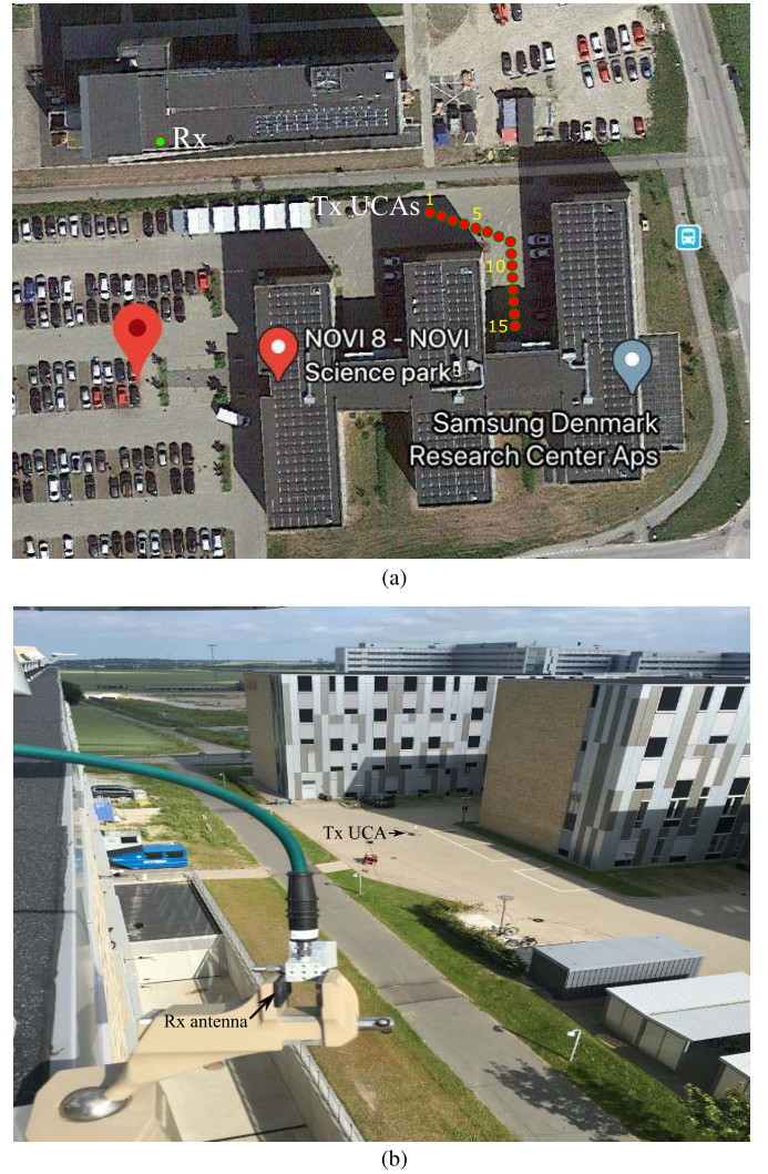
Fig. 4. (a) Aerial view and (b) photograph of the environment for the outdoor measurement campaign conducted at Aalborg University. Measurements from transmit antenna location number 7 are presented in this article.
