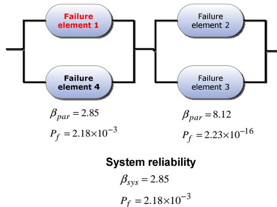
Figure 8: System reliability with damaged element 1
