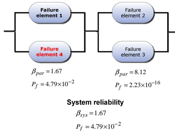
Figure 7: System reliability with damaged element 4
