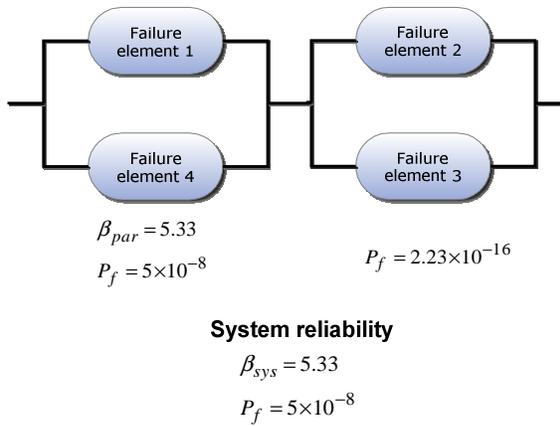
Figure 5: System reliability of the intact structure
