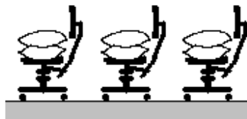
Figure 2 Side view of floor strip at midspan. Three swivel chairs each carrying 80 kg ( m = 240 \text{ kg} ).
