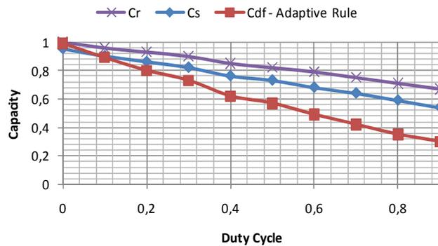
Figure 16. Capacity vs. Channel Occupation, with mean correlation 0.2 and 20 cluster nodes
