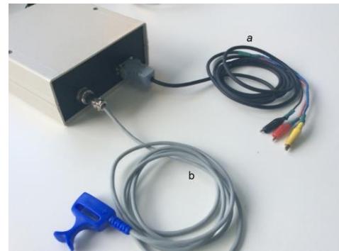
Fig. 7 The final prototype of the developed device. (a) Recording cable. (b) Stimulation cable.
