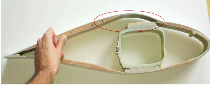
Fig. 1.10: Buckling can cause high peeling stresses and thereby skin debonding. Adapted with permission from Find Mølholt Jensen, Bladena.
