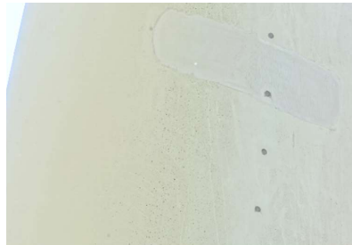
Fig. 1.15: Crack in panel repaired with D-string solution. Adapted with permission from Find Mølholt Jensen, Bladena.
