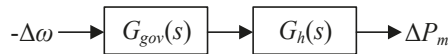
Figure 1. Open-loop system for a governor and a turbine. Symbols: \omega , rotating speed; G_{gov} , governor transfer function; G_h , turbine transfer function; P_m , mechanical power.
