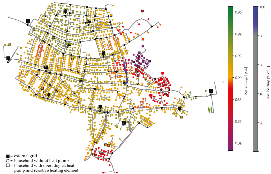
Figure 11. Synthetic low voltage grid of the town with 171 geHPs and 76 eHPs (case 3—mixed). Line overloads and bus voltages at time step with the lowest bus voltage, prior to sectioning point optimization and grid extension. geHPs are not represented in the figure.
