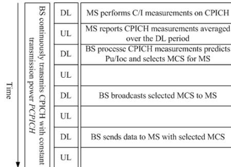
Figure 3: Obtaining SIR and MCS selection algorithm cycle.
